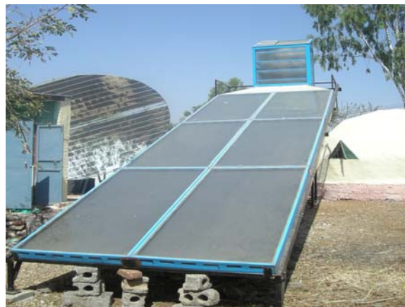
Solar drier constructed and erected by students
