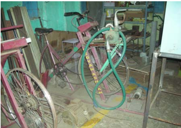
Improved cycle with a motor attached for generating electricity
